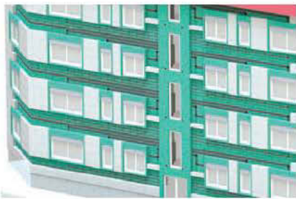
Model shows the wiring and pipes integrated in the façade of a demonstration building from the 1950s in Frankfurt, Germany. ©Fraunhofer ISE
