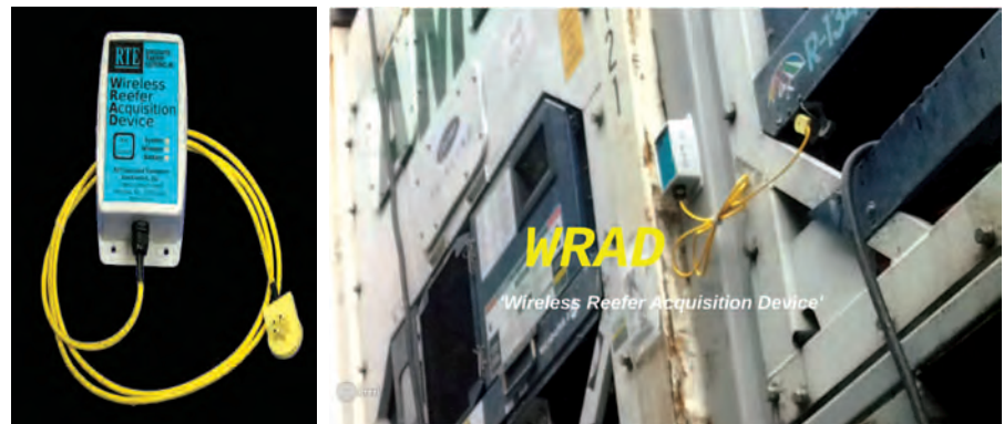
Fig. 4: Wireless Reefer Data Acquisition Device (WRAD) developed by RTE...
