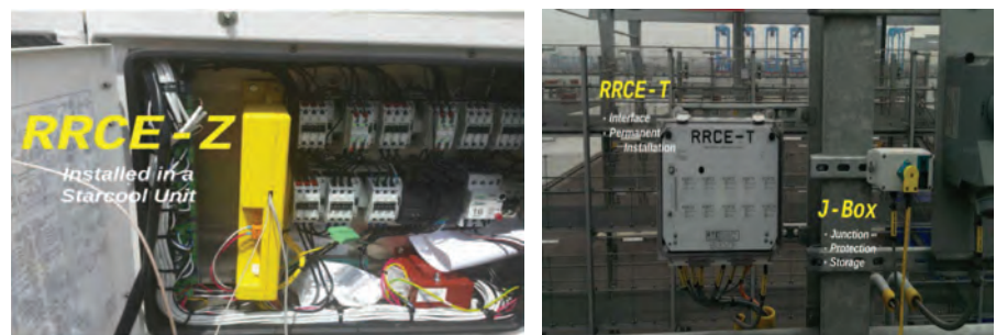
Fig. 4: Wireless Reefer Data Acquisition Device (WRAD) developed by RTE...
