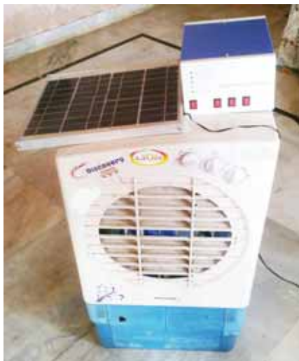
Solar Air Cooler
