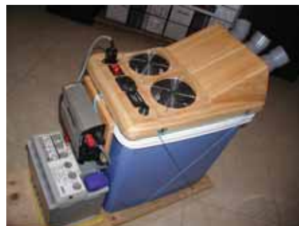
Solar Air Conditioner
