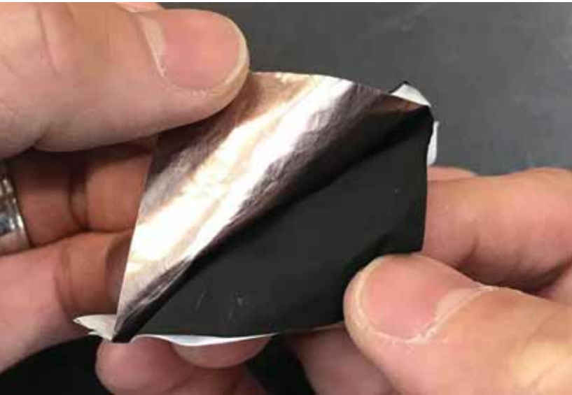
Two layers of material with different abilities to release heat energy are stacked together and sandwiched between layers of polyethylene. (Image credit: Yi Cui Group)
