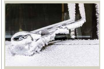
Unobstructed visibility in any weather Even if the windscreen wiper of the ICE 4 is iced, it still ensures a clear view for the driver: The field of view is free of streaks and the windscreen nozzles are fully functional despite the icy temperatures. But not all tests are conducted by sight alone: Experts from Siemens and Rail Tec Arsenal (RTA) have installed around 500 highly sensitive sensors in the train cars to precisely monitor how the train reacts to heat, cold and ice.
