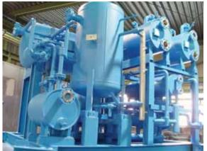
Maintenance: To ensure fairly noncorrosive solutions for a long period of time, it is very important to monitor the inhibitor concentration and replenish the inhibitor as necessary. For this, the pH reading should be regularly recorded followed with periodical analysis of solution sample. This systematic approach also will prevent indiscriminate addition of inhibitor, which is also very harmful.
