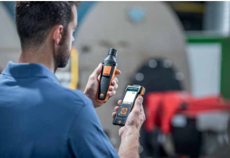
Testo-440 - CO level measurement with Bluetooth probe
