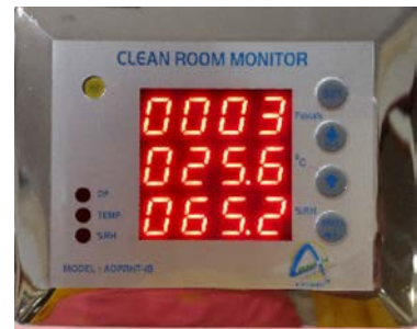
Series ADPRHT - Aerosense differential pressure/RH/Temp for clean room applications.
