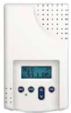
Figure 4 (above) Shows a Telaire make Dewpoint Sensor used for moisture removal/prevention of mold formation...
