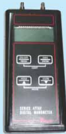
Series 477AV Dwyer Handheld Digital Manometer
