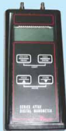
Series 477AV Dwyer Handheld Digital Manometer
