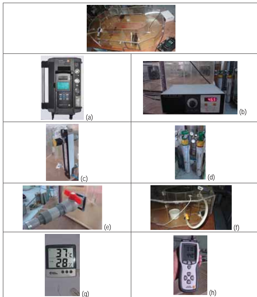
Figure 1. Environmental Chamber and its Equipments... Fig (a) is the Flue Gas Analyzer, (b) Thermostat (Temperature controller), (c) Rotameter, (d) The SO 2 , NO 2 Aluminium Cylinders, (e) Outlet, (f) Probe of Flue Gas Analyzer, (g) Relative Humidity & Temperature Traceable Instrument, (h) Hot Wire Anemometer.
