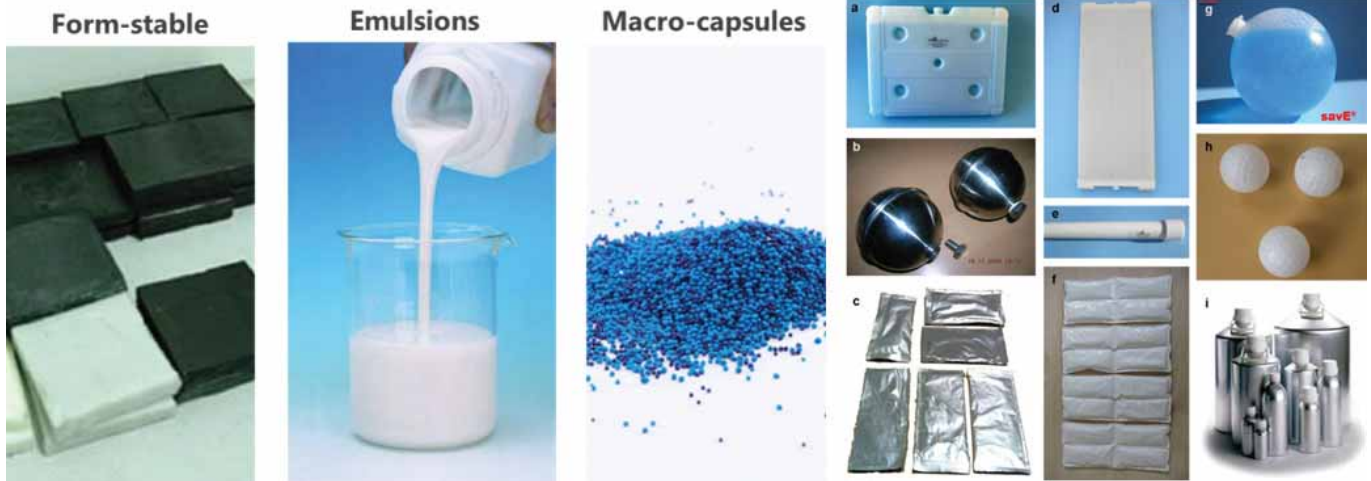
Figure 5 (a) New commercialized PCMs for building applications; (b) Encapsulation technology available: a. HDPE Polymer Thermotabs; b. Stainless Steel balls; c. High barrier Aluminum foil; d. HDPE extrusion profiles; e. HDPE pipes; f. PET film; g. HDPE 70mm balls; h. HDPE 25mm balls; i. Aluminum bottles
