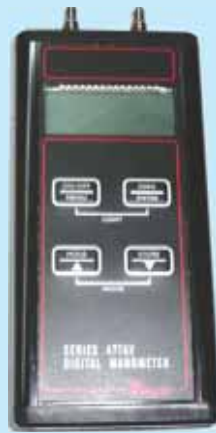
Series 477AV Dwyer Handheld Digital Manometer
