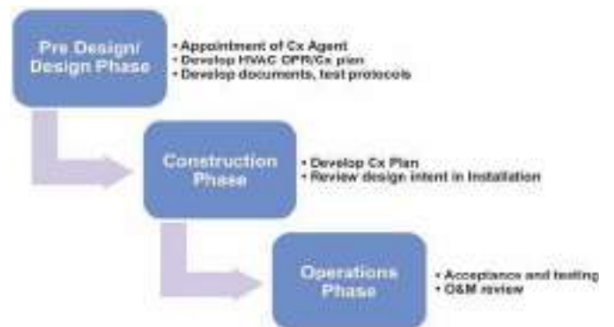
Fig. 1: HVAC Commissioning Process Overview
