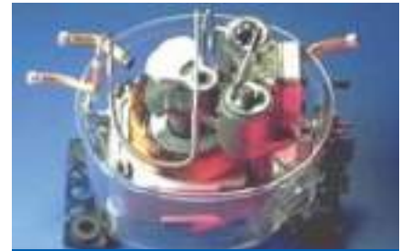
Fig. 8: Cut-away Section of a Multi-voltage compressor
