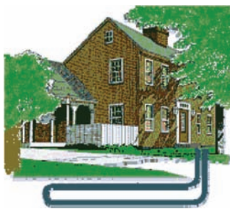
Fig. 25: Horizontal energy systems
