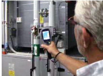
Björn Blomgren demonstrates the use of the FLIR i5 thermal imaging camera...
